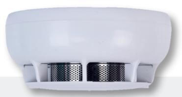
TFD-1271 and TFD-1270 detectors are uses combination of optical and heat detection technologies to sense fire and it can be connected two-wired loop circuit carrying both data and power. It uses FlashLink communication protocol to communicate Teknim Addressable control panels.
